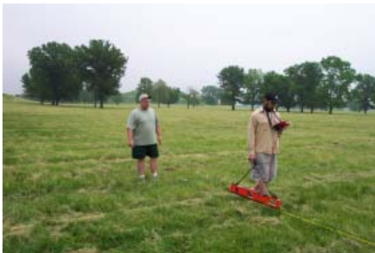
Figure 1. Earth conductivity survey in the West Palisade area using a Geonics EM38 earth conductivity meter.
